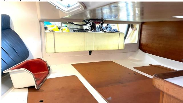
2. **Locate Ideal placement for the sensor!** Flat, smooth, far to the rear (port side) so it can't be knocked around by locker goods.
