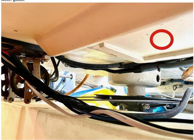
3. **Fabricate mounting block (plastic/starboard) for connection to radial drive wheel** Then bolt it on using existing holes in the radial drive wheel.
